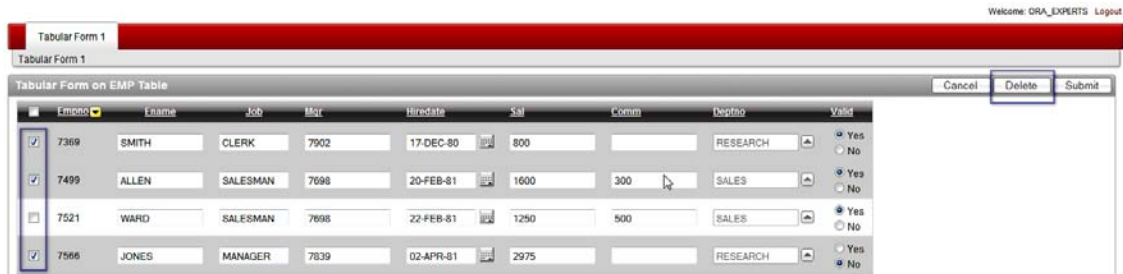
Figure 3-17. Tabular Form—deleting records using custom process
